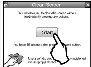
Step 4. The touch screen will be disabled for 10 seconds. Clean the bare screen or the protective film using a soft dry cloth or a cloth moistened with Isopropyl Alcohol. Avoid chemical cleaners and solvents which may damage plastic components.
