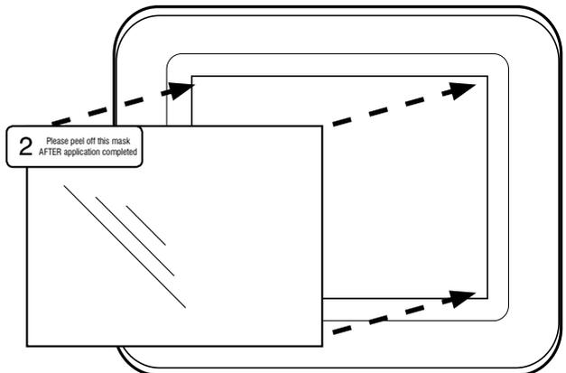
STEP 4. Use the green tab to peel off and discard the topmost layer of the film. Your Navigator is now ready for use.
